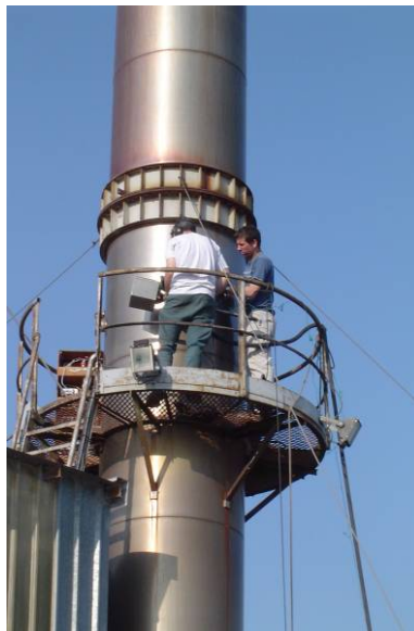
Photo 4 - Location of the sampling zone for the analyses of fumes at coating plants.
