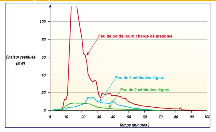
The energy produced by a light car in fire is ten times lower then by a heavy truck
