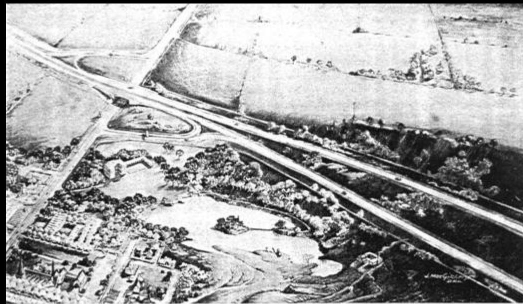
PLATE 31.—A typical grade separation, access roads, and toll booths for a four-lane road.
