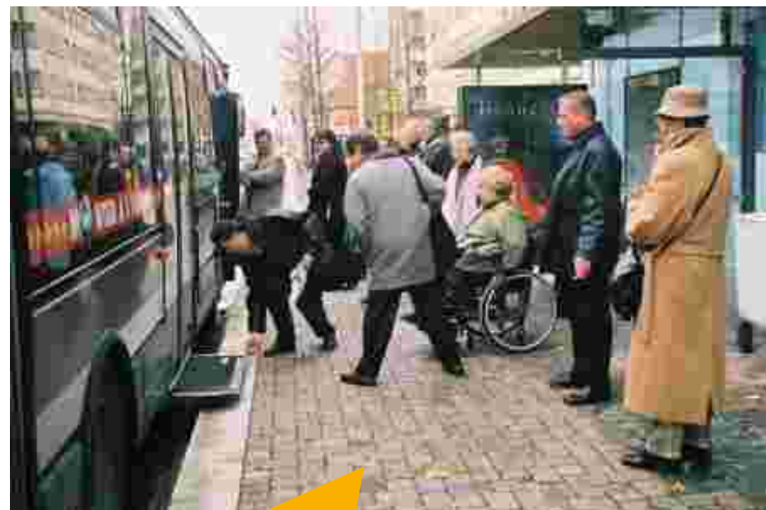
Raised bus stop and low-floor vehicle
