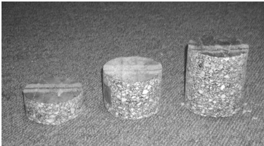
Figure 4. Core samples from failed test sections
