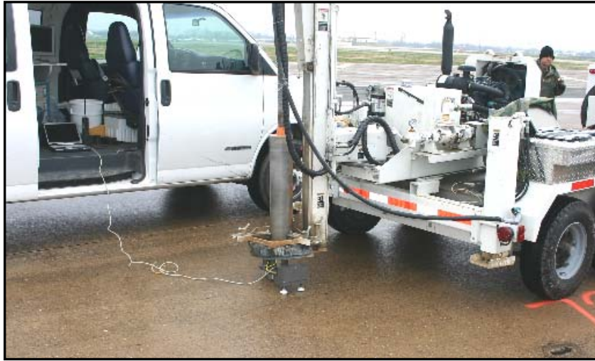
Figure 2 – PSPA testing at the core hole location.
