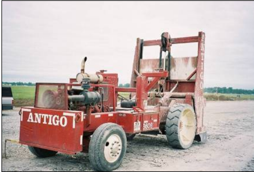
Figure 6. Guillotine Style Breaker
