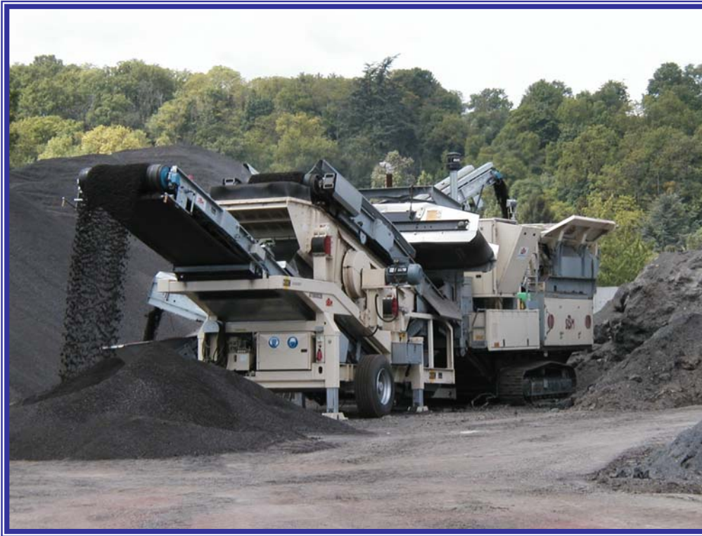
[figure 5: SBM crusher in action, crushing surfacing aggregates]
