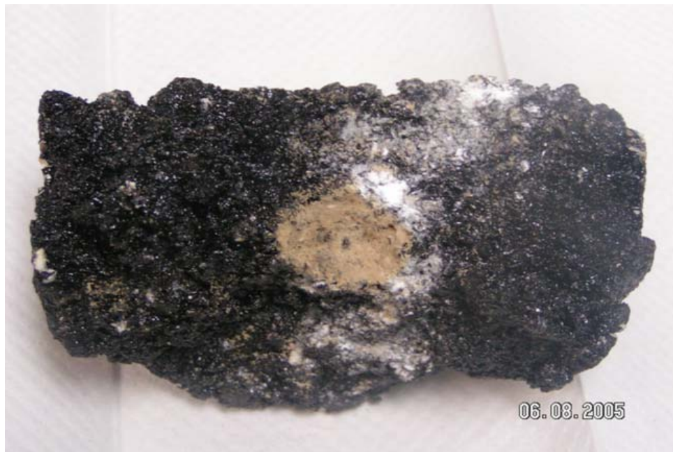
Figure 7. Removed sample of HMA showing clayball.
