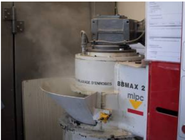
Mixing in laboratory: very little emission of dust, bulk material before Gyratory Shear Compaction (PCG) test, absence of fumes, some light vapours.
