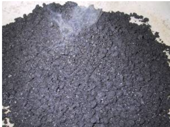
Mixing in laboratory: very little emission of dust, bulk material before Gyratory Shear Compaction (PCG) test, absence of fumes, some light vapours.
