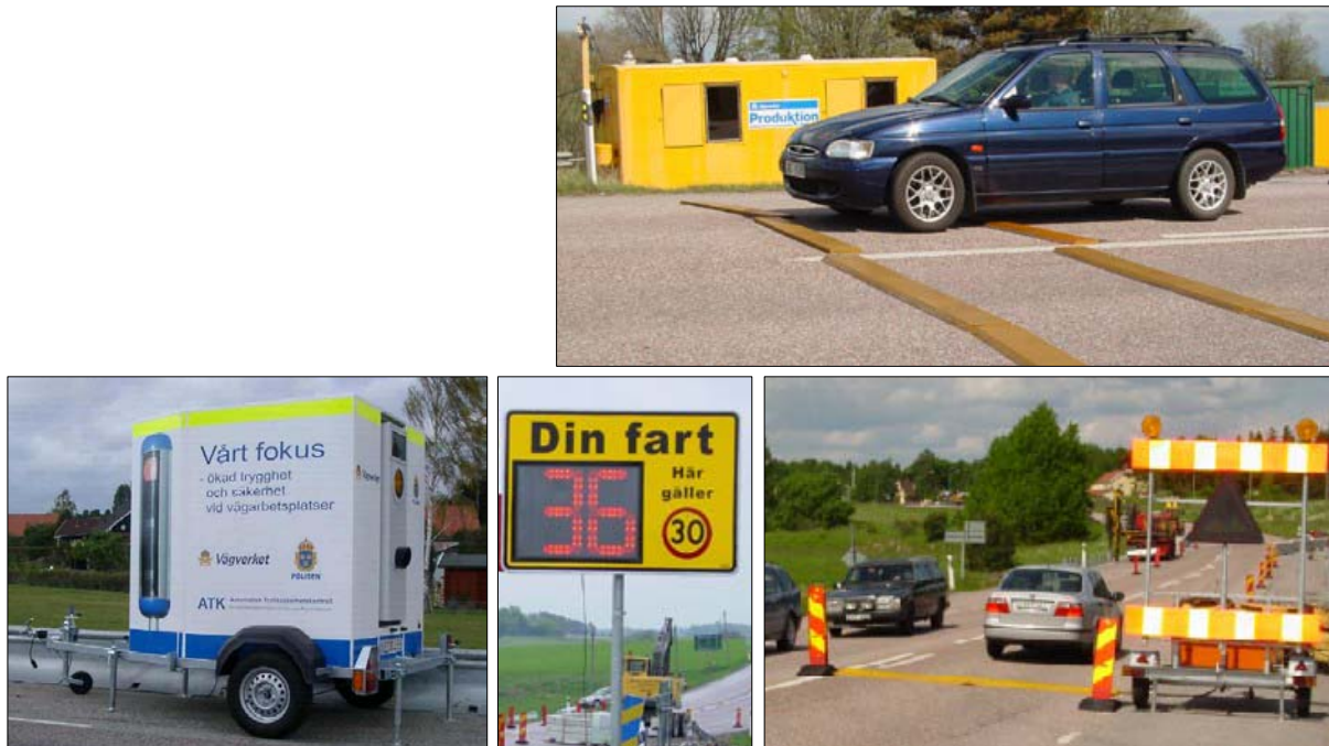
Figure 1 - Tested products. Mini speed bump (top right), mobile police speed surveillance camera (bottom left), speed display (bottom centre) and active mini-bump (bottom right without flashing lights).
