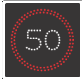
Figure 7 - Example of a VMS. The pixels in the sign can be produced using fibre optics or light emitting diodes. This LED sign was used in the project, for instance, to evaluate the effect of a VMS displaying the recommended speed.
