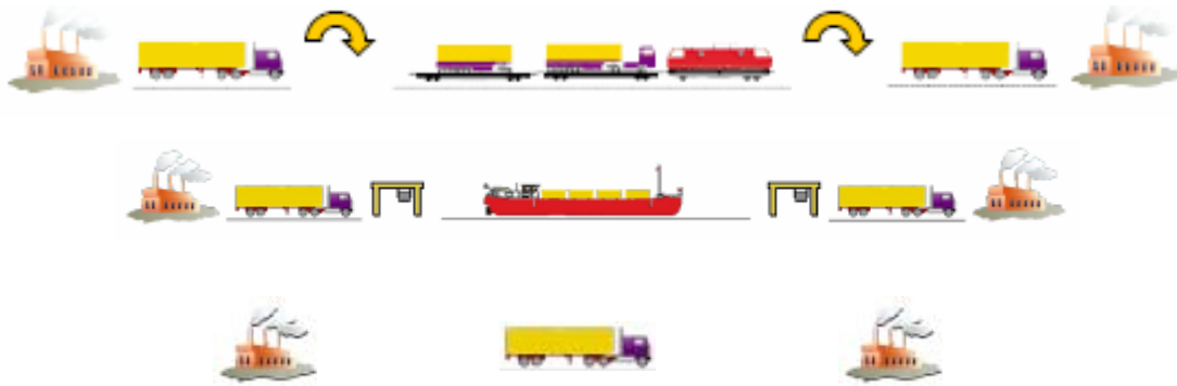
Figure 1 – Transport chain for a roll-on/roll-off railway or seaway compared with road transport
