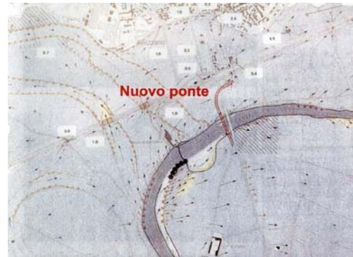
Picture n° 4 – Plan of the area of Felizzano, with the flood surface reached by the Tanaro and the placing of the new bridge on the main road 77.
