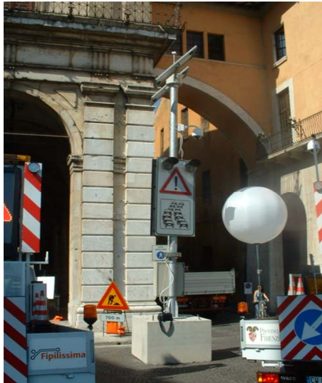
“Figure 4 – Signalling queues: rotating panels that can be utilised by remote control and equipped with video-cameras”
