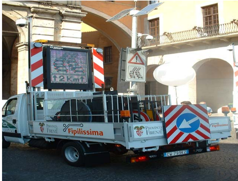
“Figure 3 – Detail of the dynamic message panel on a truck”
