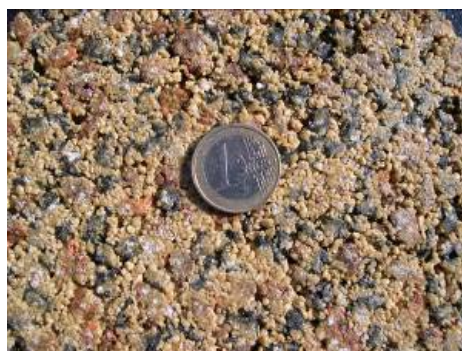
Photo 2- Plant-based binder mix with the natural colour of the aggregate
