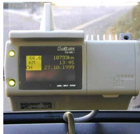
Figure 15: HVF System Size and On Board Unit (Rapp Trans AG)
