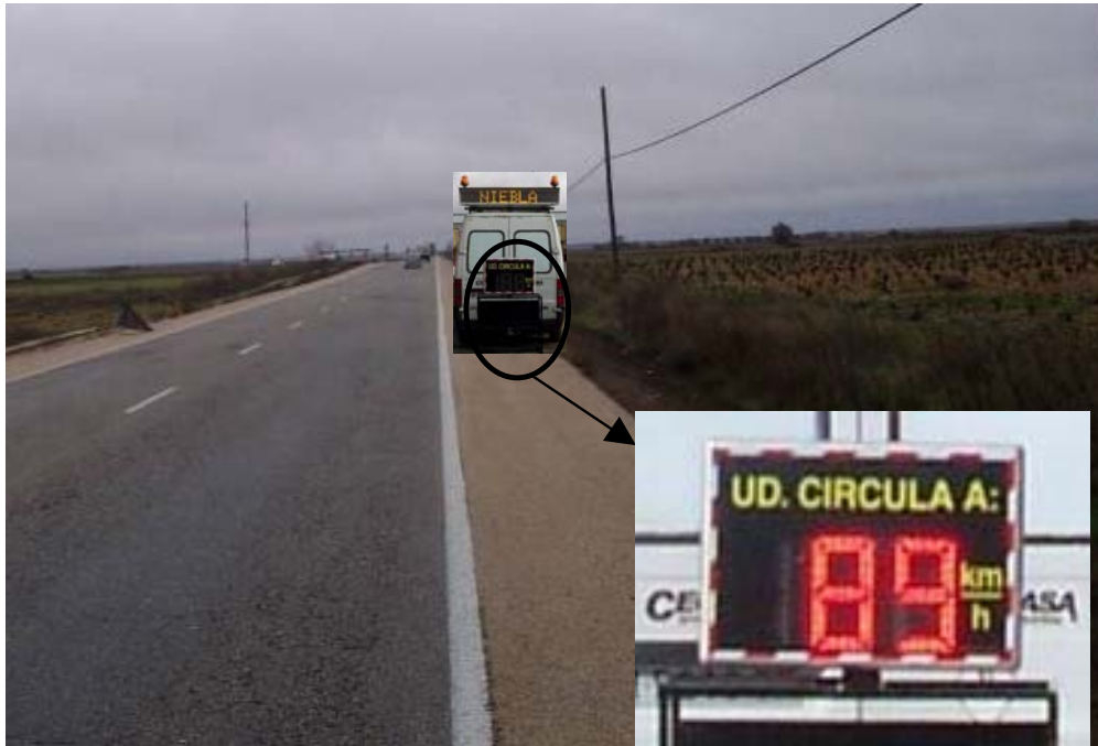
FIGURE 4 - Reinforcement mobile variable message sign used in AAWWS pilot tests equipped with a radar speed detector
