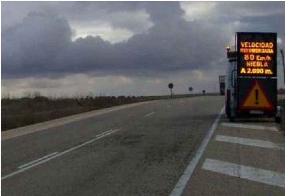
FIGURE 3 - Pre-warning mobile variable message sign used in AAWWS pilot tests
