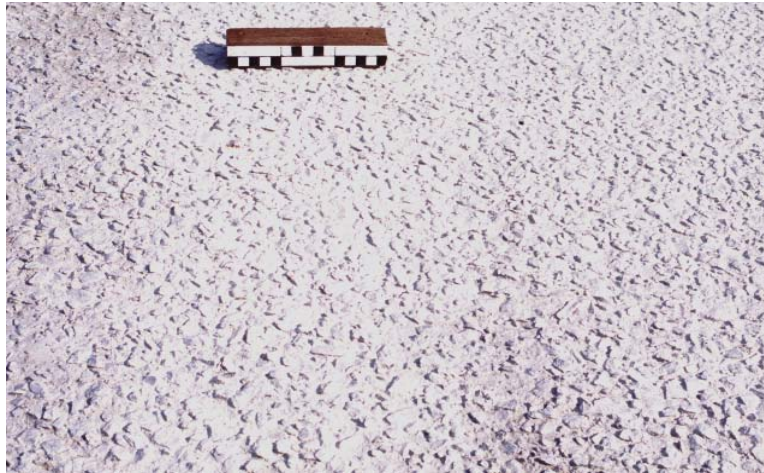
Figure 3 – Appearance of a surface after aggregate exposure
