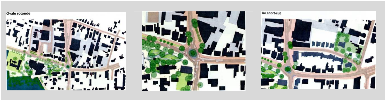
Figure 10 – Doorn: oval-shaped roundabout, by-pass and shortcut road
