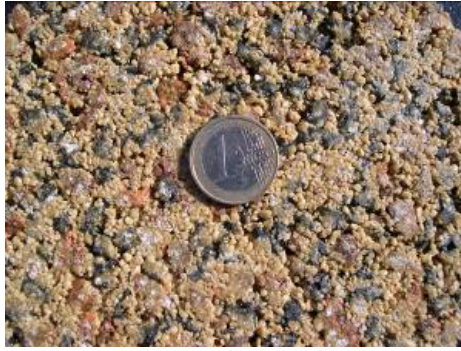
Photo 7 – asphalt mix with plant-based binder showing the natural color of the aggregates
