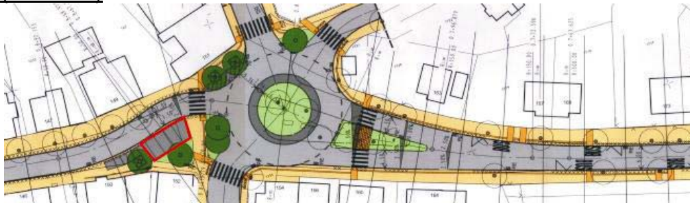
Picture 5: Detailed design „Sight obstructions at pedestrians caused by parking vehicles“
