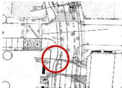
Picture 15: Detailed design „Lacking/inadequate measures to prevent illegal parked cars”
