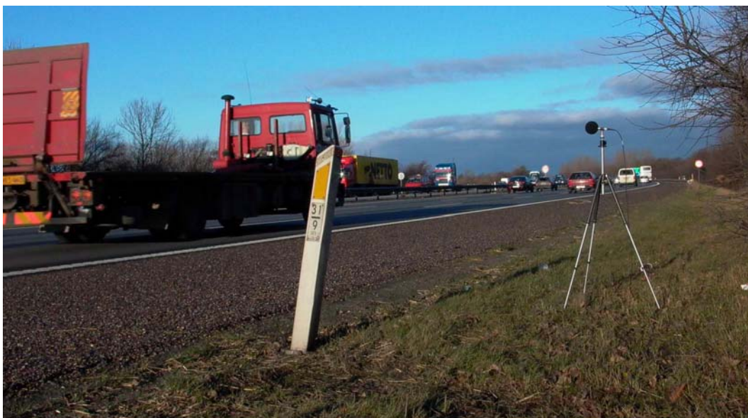
Figure 13 – Typical microphone setup at the SPB noise measurements at the test sections at M10.
