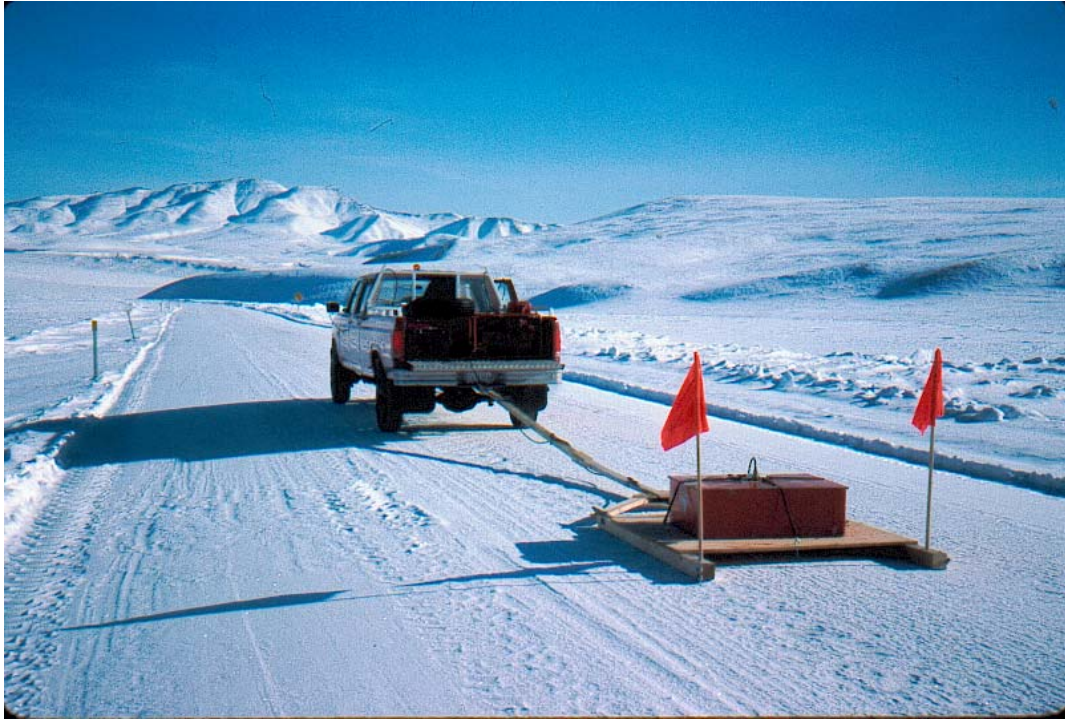
Figure 2 – Ground Penetrating Radar Survey, Dempster Highway
