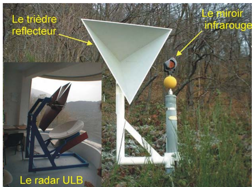
Figure 9 - Distance measurements by radar: on the left, the radar sheltered in a cabin located on the southern slope; a trihedron reflector for the radar measurements, beside a mirror for the infra-red measurements.
