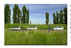
On the track land, it is envisaged to implement test benches, enabling to qualify specific equipments. It was decided to implement a first bench to test on-board perception sensors, allowing repetitive tests in a configurable environment, including lighting and meteorological situations. The test bench will enable to qualify new on-board sensors for obstacle detection.
