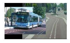
The project comprises the development of an aid to longitudinal guidance for the buses of TEOR type, using the z profile of the route. An interface will be available for the driver, indicating the driving condition and potential suggestions to reduce fuel consumption, to improve the passenger comfort, and to cross intersections
