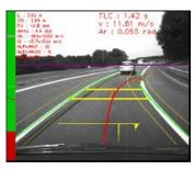
The main objective is to prevent ram off roadway accidents. The image processing team works concern the development of measurements: lateral discrepancy, TLC, tangent point... Partnership: CNRS, INRETS-LCPC, Renault, PSA.
