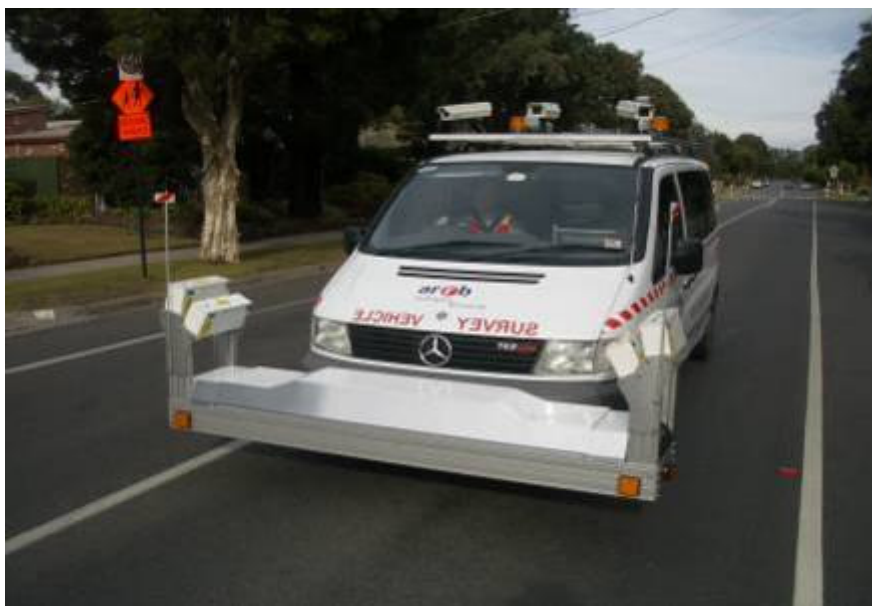
Figure 3: Star-ratings data are collected by specially equipped vehicles
