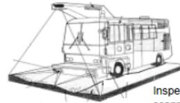
Inspection of road surface by laser scanner and scan image
