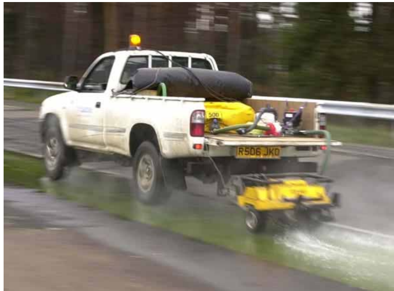
Figure 7 - Testing of skid resistance in wet conditions
