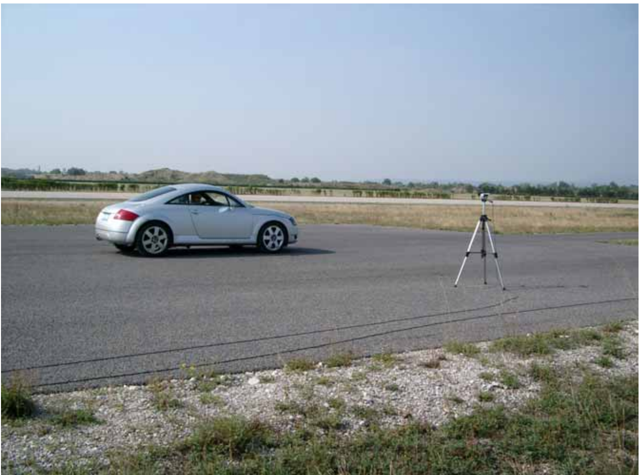
Figure 3 – Car pass-by noise measurement setup according to ISO 362.
