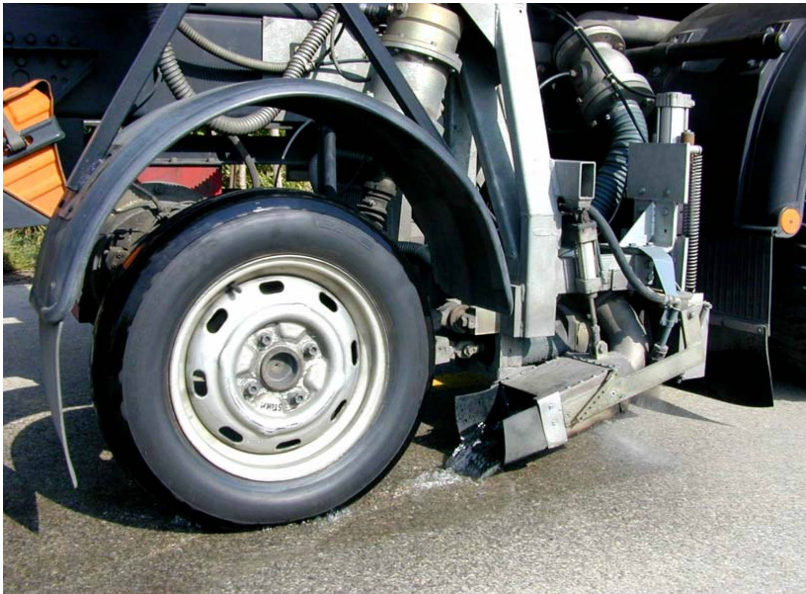
The ribbed PIARC test tyre on ROADStar (Austria)
